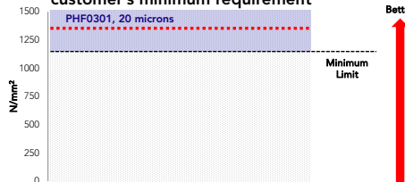
Figure 5. Elastic modulus in machine direction of 20 micron plain film made of EVALENE® PHF0301 vs. customer's minimum requirement
