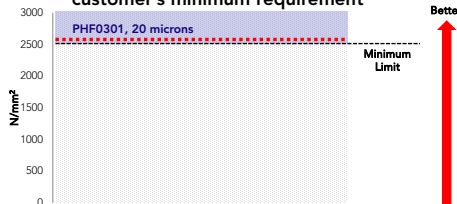
Figure 6. Elastic modulus in transverse direction of 20 micron plain film made of EVALENE® PHF0301 vs. customer's minimum requirement
